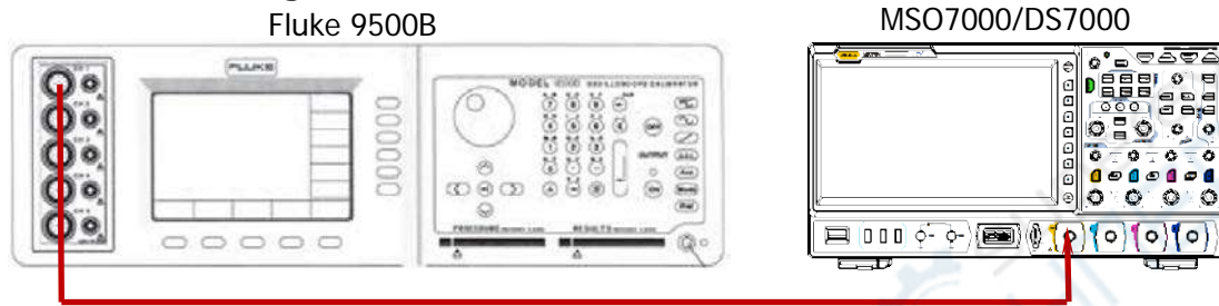
Figure 2-1 Impedance Test Connection Diagram
