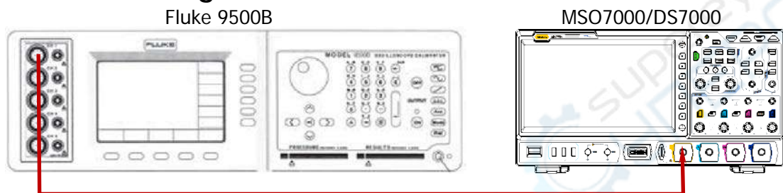
Figure 2-5 Timebase Accuracy Test Connection Diagram
