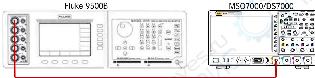
Figure 2-3 Bandwidth Test Connection Diagram
