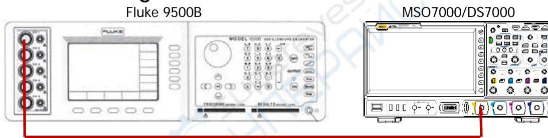
Figure 2-4 Bandwidth Limit Test Connection Diagram
