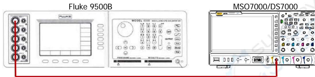
Figure 2-2 DC Gain Accuracy Test Connection Diagram
