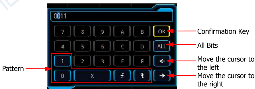
Figure 5-6 Virtual Keypad for Pattern Setting
