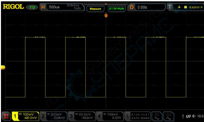
Figure 4-3 Waveforms after 128 Times of Averaging
